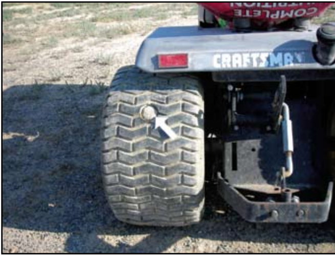
The hole (by arrow) that was cut to fill the tires with concrete.
