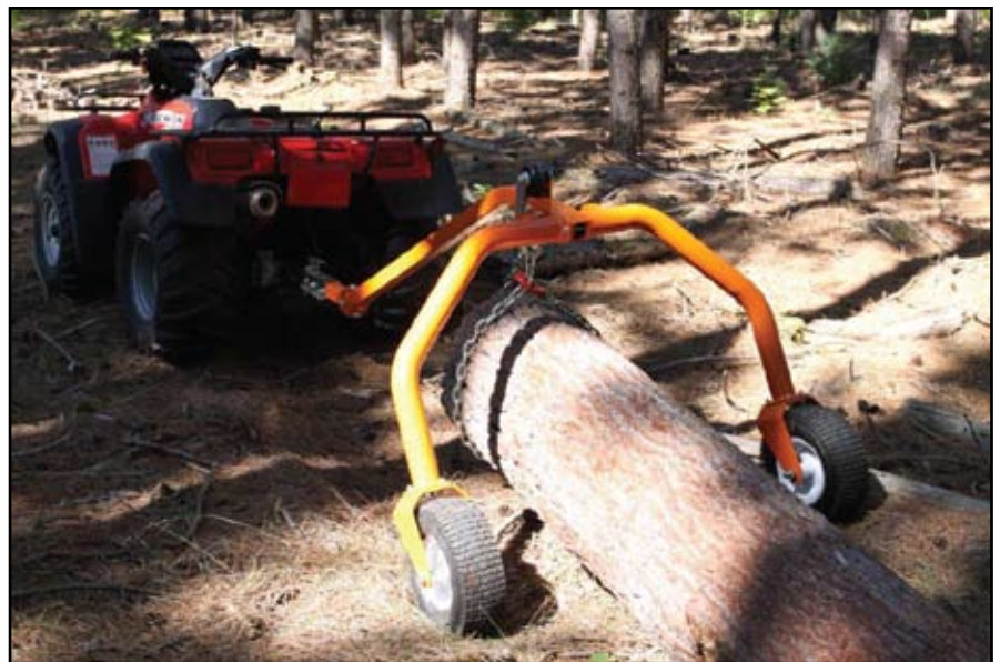
Hauling a log with an ATV arch.
