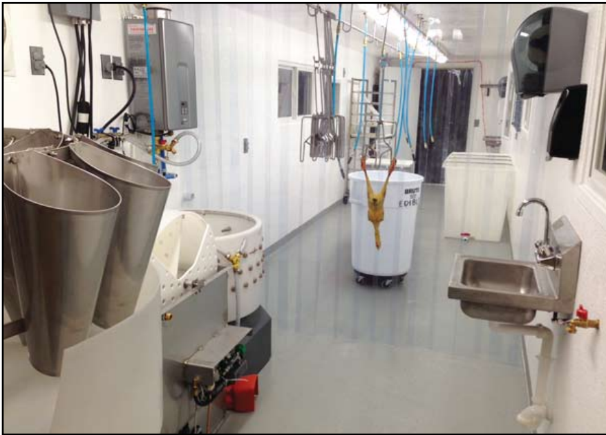
Left: David Schafer built an entire USDA chicken processing plant inside of an 8' x 40' shipping container.
